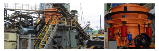
Furthermore, the liner change cycles are 3-4 months as normal cone crusher liner replacement. Simply by replacing liners, various on-spec products from coarse to fine aggregate can be achieved.
